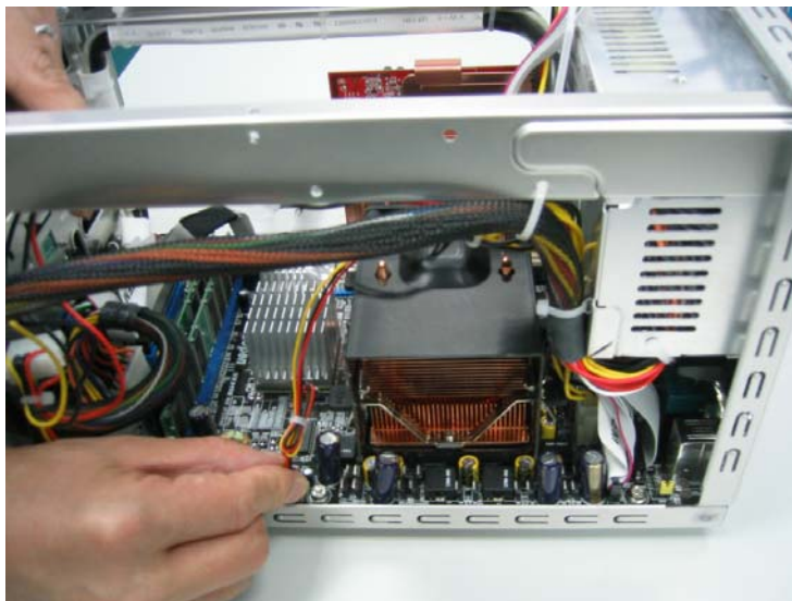
Fig 6 Plugging in the fan power cable
